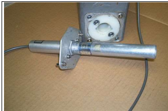
Victoreen Neutron Survey Meter Model 488A 1950's
