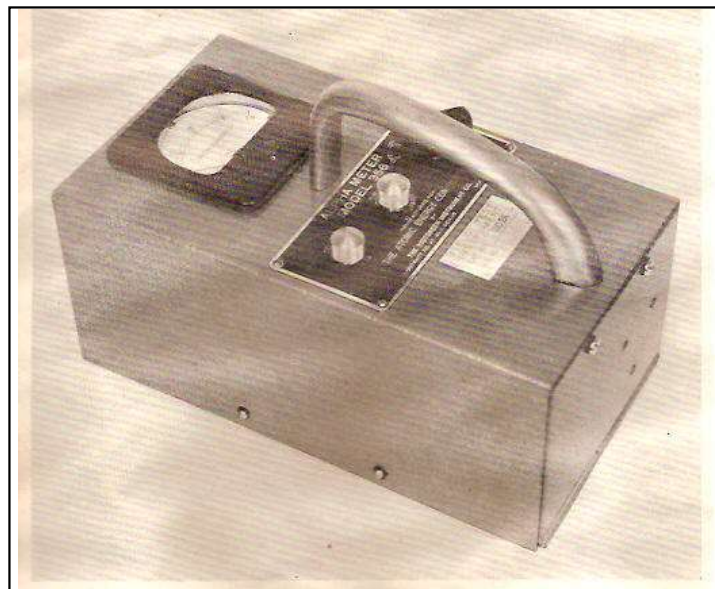
Victoreen Alpha Survey Meter Model 356 1948
