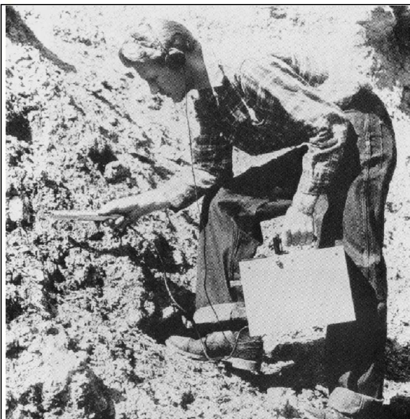
H.R. Hanson of Victoreen Instrument Co. checking portable survey meter, a Model 263 Doc 1945, from Health Physics: A Backward Glance by R. Kathren and P. Ziemer, 1980.
