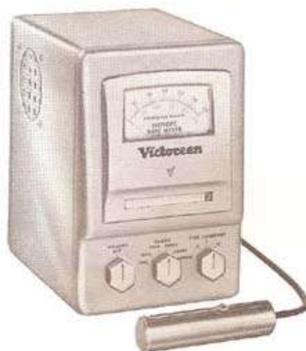
Model 524 Isotope Ratemeter with probe, 1B85 tube, and Instruction Manual . . . . . $375.00
